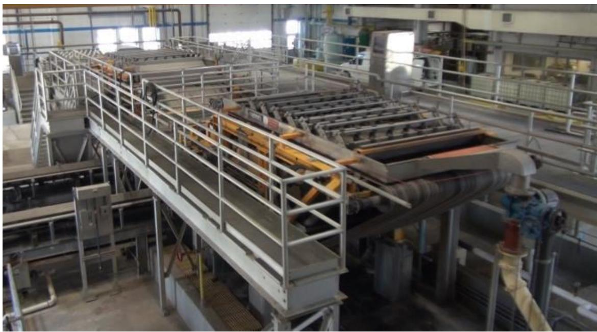
Polymer is mixed with sludge and fed to the equipment
