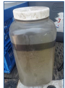
A sample collected from the sanitary sewer on August 2 with at least one inch of floating oily material.
