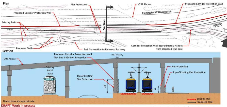
Current project design includes pier protection on both sides of the LRT under I-394
