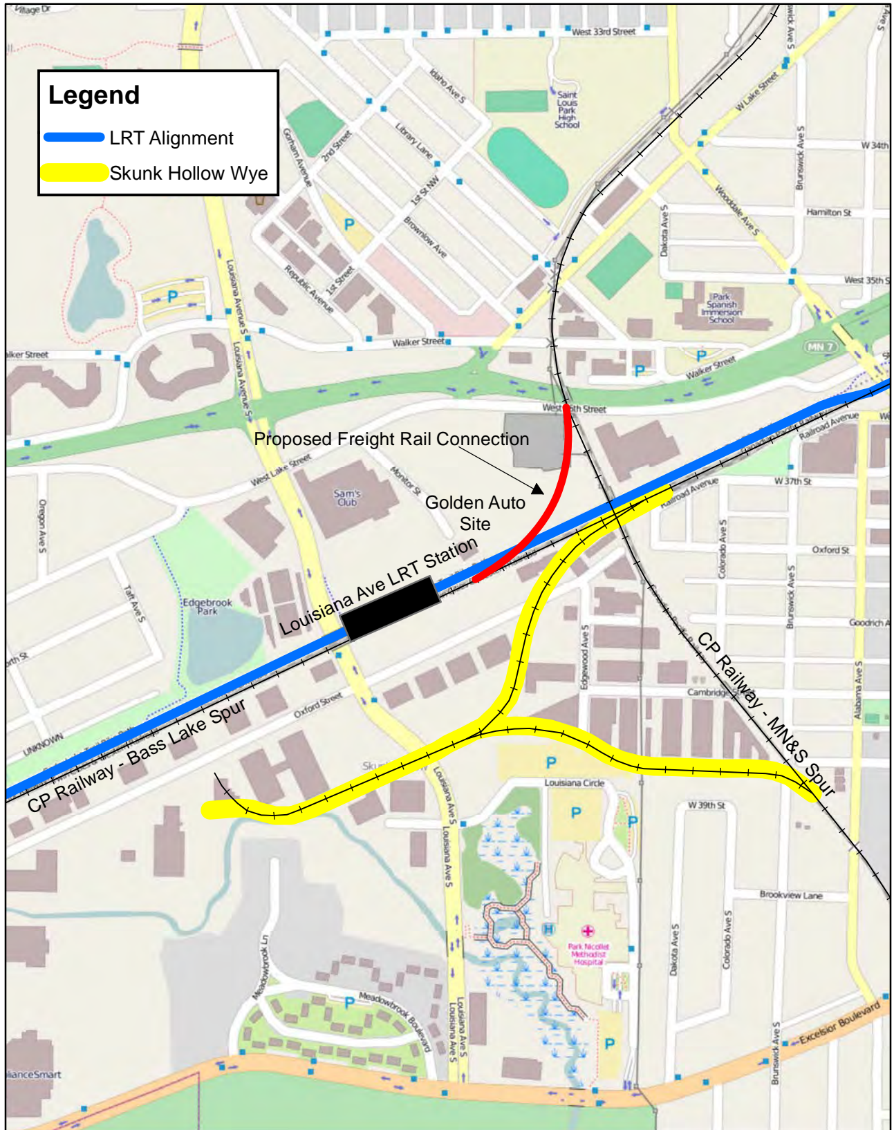
Figure 2. Relocation Alternative Skunk Hollow Wye Track and New Connection - Bass Lake Spur to MN&S Spur
