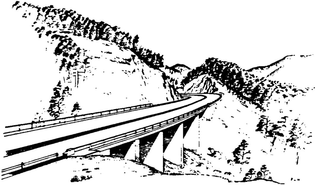
Removing a residual piece of rock between the freeway and a natural slope can lead to smoother landscape design and can open up vistas which are otherwise obscured
