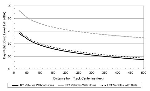
Projected Bottineau LRT Noise Exposure (No Shielding, 55 mph Train Speed, Ballast & Tie Track)
