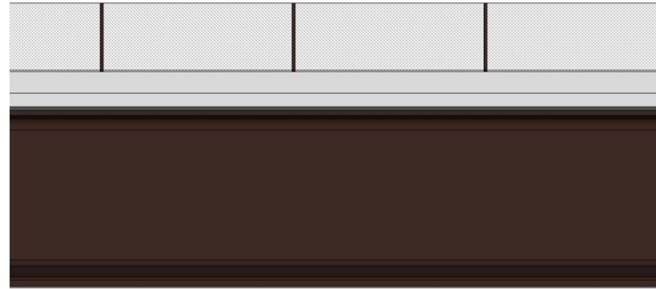
Elevation of bridge with T.H. 212 color palette with diamond mesh safety rail.
