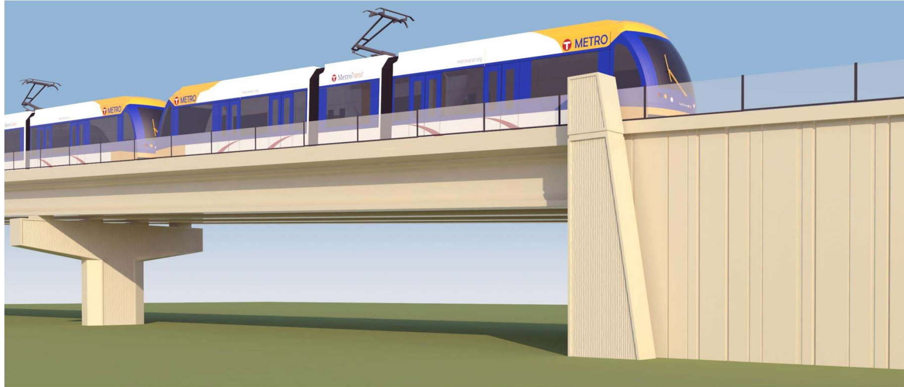
LRT bridge pier with base pilaster and pinnacle
