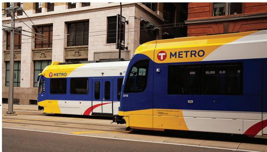
Weighing in at 6,000 pounds lighter, the new Siemens' light rail vehicles (pictured front) are more energy efficient than the light rail vehicles (pictured back) purchased for Hiawatha LRT.
