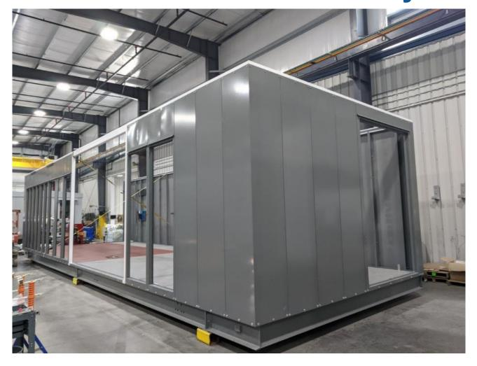
This is the first Traction Power Substation (TPSS) to begin assembly and will be delivered to the project for use at the Franklin O&M Facility in support of the SWLRT LRVs
